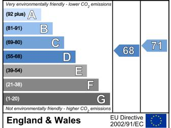
The environmental impact rating is a measure of a home's impact on the environment in terms of carbon dioxide ( $CO_2$ ) emissions. The higher the rating the less impact it has on the environment.
